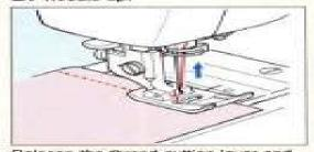
Release the thread cutting lever and the needle will go up, and the upper and bobbin threads are cut. The needle stops in the up position.
