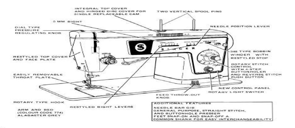
Servicing instructions for 478 Machine apply to the 477 with the exception of ADJUSTING THE CAM STACK as shown on page 55.
